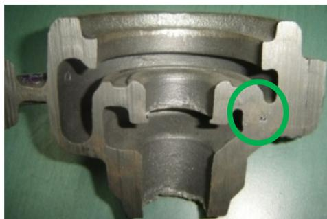
The hotspot indicated by solidification contour exactly matches with the shrinkage porosity found in actual casting.
