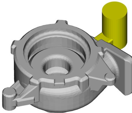
Solidification simulation analysis shows feeder is slightly undersize and there is a clear isolated hot spot inside casting. This is primarily due to the Y-junction in the casting design.
