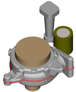
Liquid fraction analysis displays all liquid metal inside the feeder and sprue at the end of casting.
