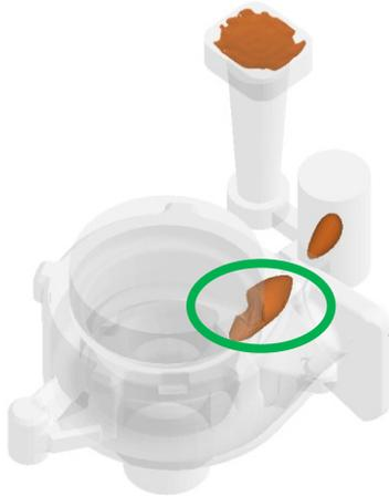
Liquid fraction analysis displays liquid metal remains inside the casting till the end of solidification. This indicates these locations can have shrinkage porosity.
