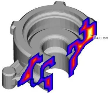
Wall thickness analysis shows a heavy section with 25 mm thickness (inscribed sphere diameter).
