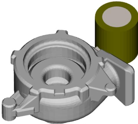
← The feeder dimension was revised to 65 mm height and 40 mm bottom diameter with an insulating sleeve of thickness 8-10 mm along with a chill (25 mm cube) below the defect zone and further analyzed for the hot spot.
