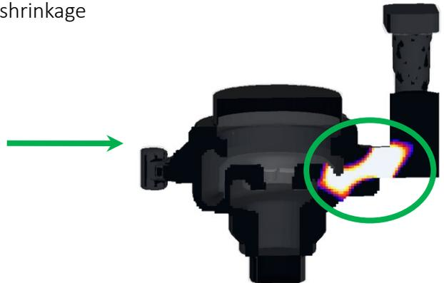
Shrinkage porosity is seen inside the feeder and neck. The lighter colour shows micro shrinkages and darker colour shows macro shrinkages.
