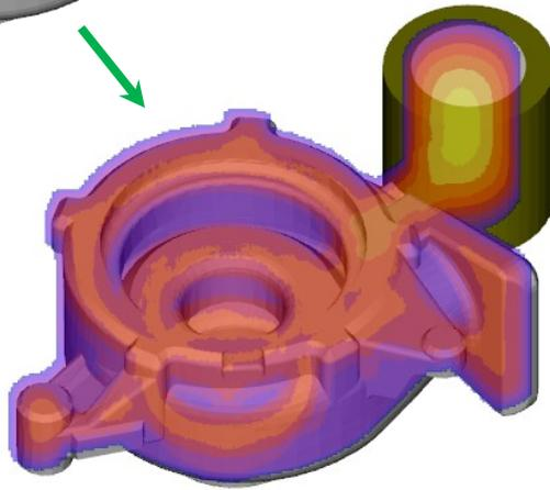
← 3-Dimensional solidification contour shows uniform temperature profile and directional solidification towards feeder.
