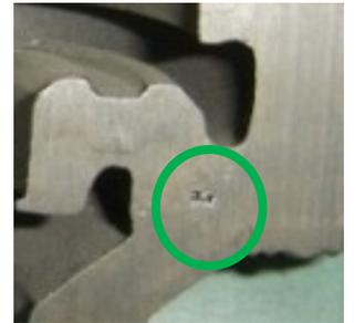
Side feeder used in the foundry (35 mm bottom diameter, 60 mm height) is correctly connected to the thickest section in casting.
